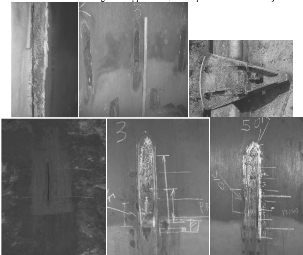
Figure 5.1: Cracks, damages and fracture of autoclave components during the service
