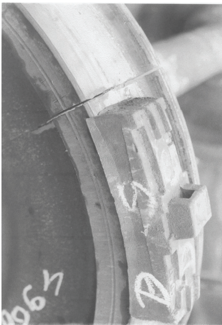
Figure 9: Fractured monoblock wheel
