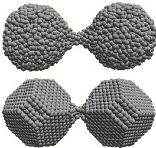
Figure 24. NIST researchers have shown that silica that are brittle in bulk exhibit ductile behaviour at the nanoscale. Computer simulations demonstrate the material extension and necking that occurs during the separation of amorphous (top) and crystalline (bottom) silica nanoparticles /26/
