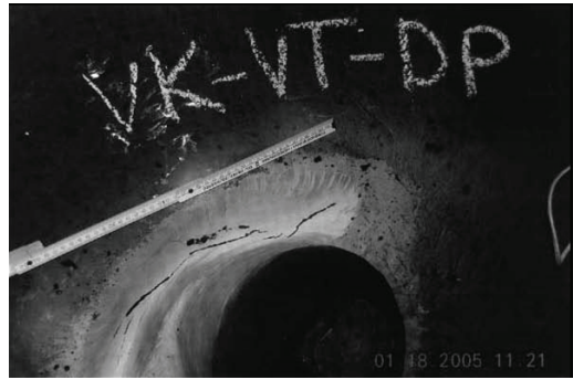
Figure 7: Indication 420 mm long obtained by dye penetrant testing
