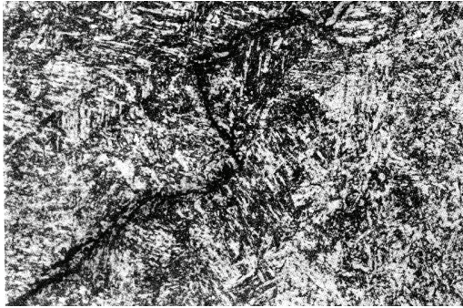
Figure 9. Hot crack in weld metal
