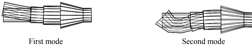
Figure 7.9: First and second mode of oscillations of the input-shaft (coupling mass 500 kg)
